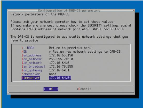
FIGURE 5: SETTING UP DAB CONTENTSERVER NETWORK SETTINGS INCLUDING NTP
