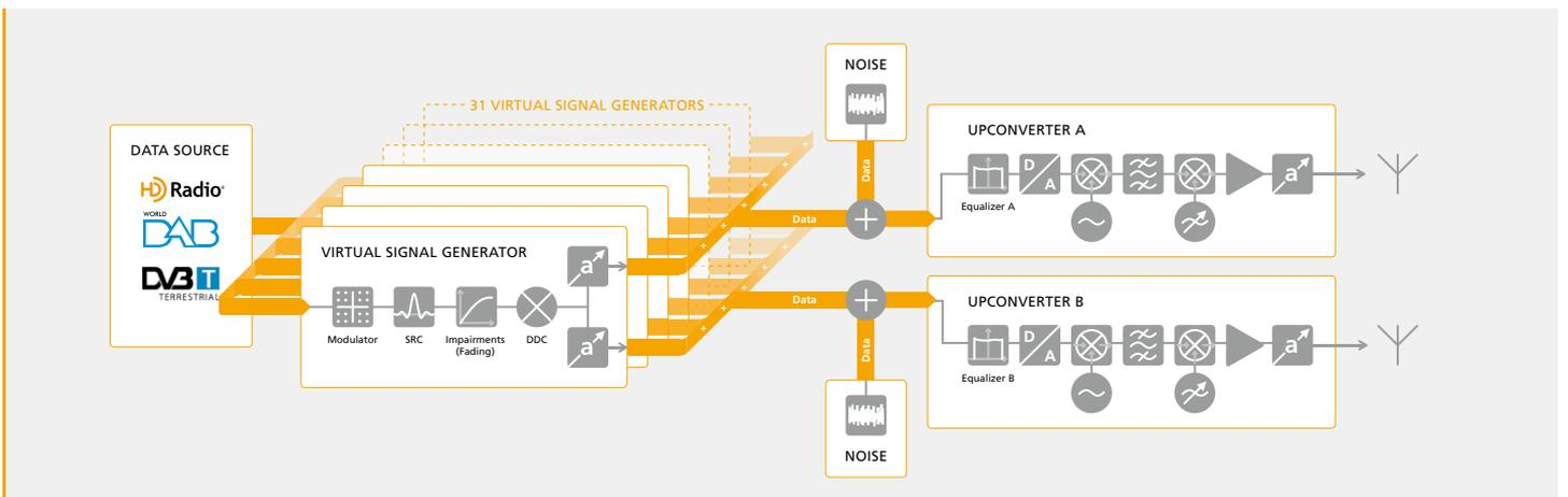
FIGURE 12: BLOCK DIAGRAM OF THE IZT S1000
