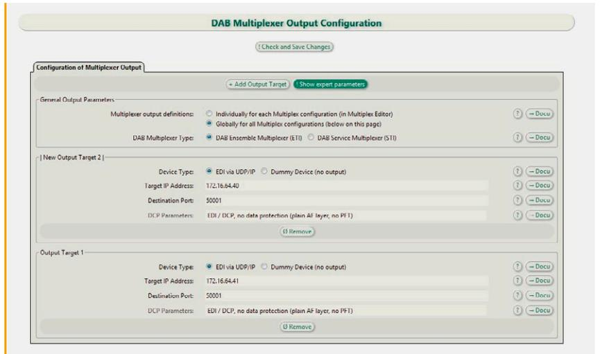
FIGURE 8: MULTIPLEXER OUTPUT CONFIGURATION OF THE IZT DAB CONTENTSERVER
