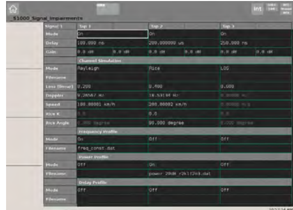
FIGURE 12: FADING CHANNEL SIMULATION
