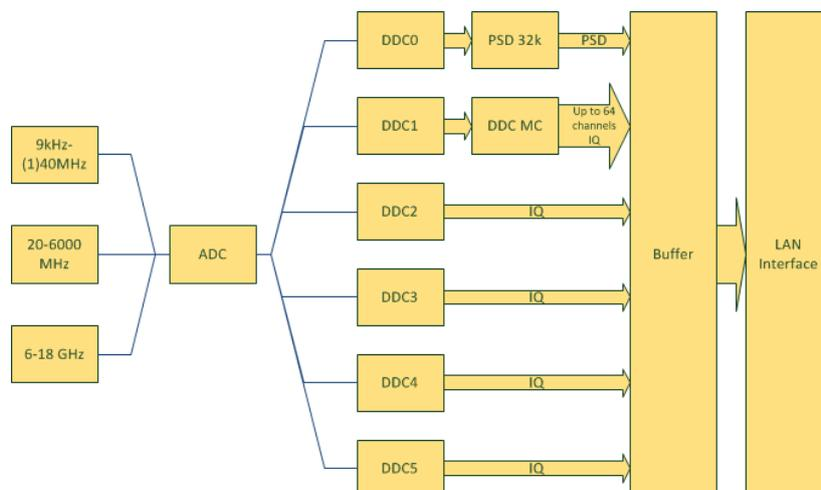
Figure 2: IZT R5040 Receiver Block Diagram
