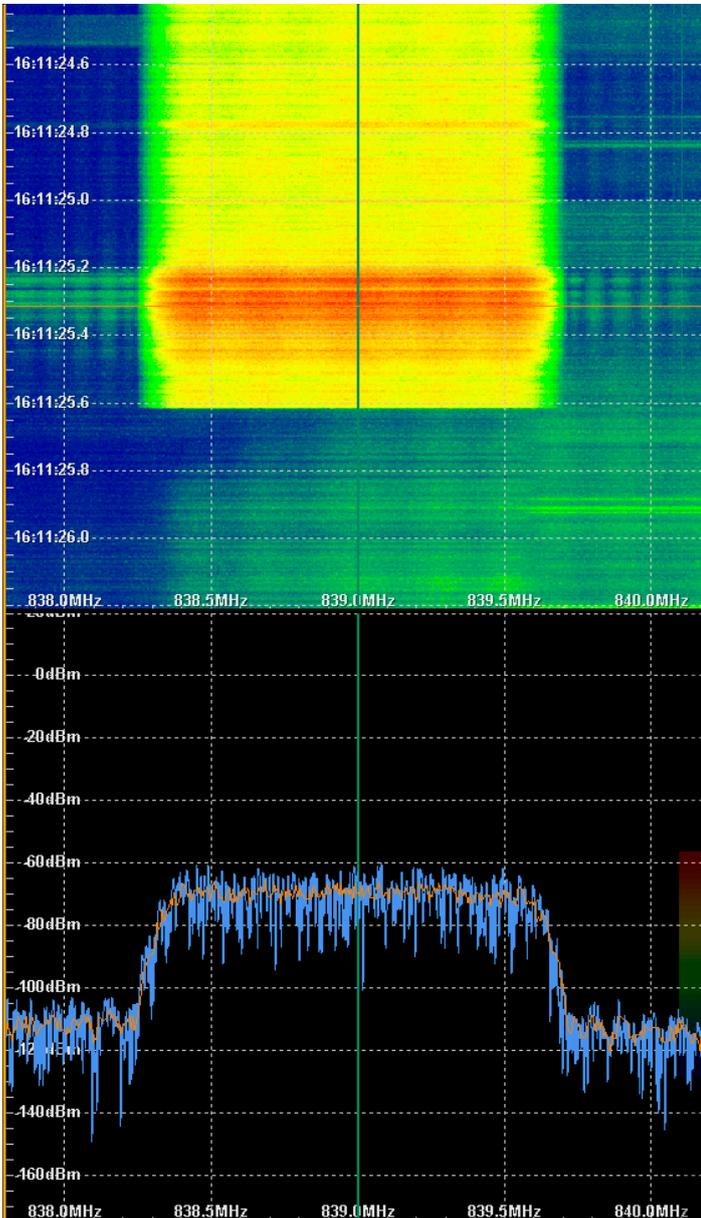
FIGURE 3: SUB-BAND MONITORING WITH SPECTRUM & SPECTROGRAM DISPLAY
