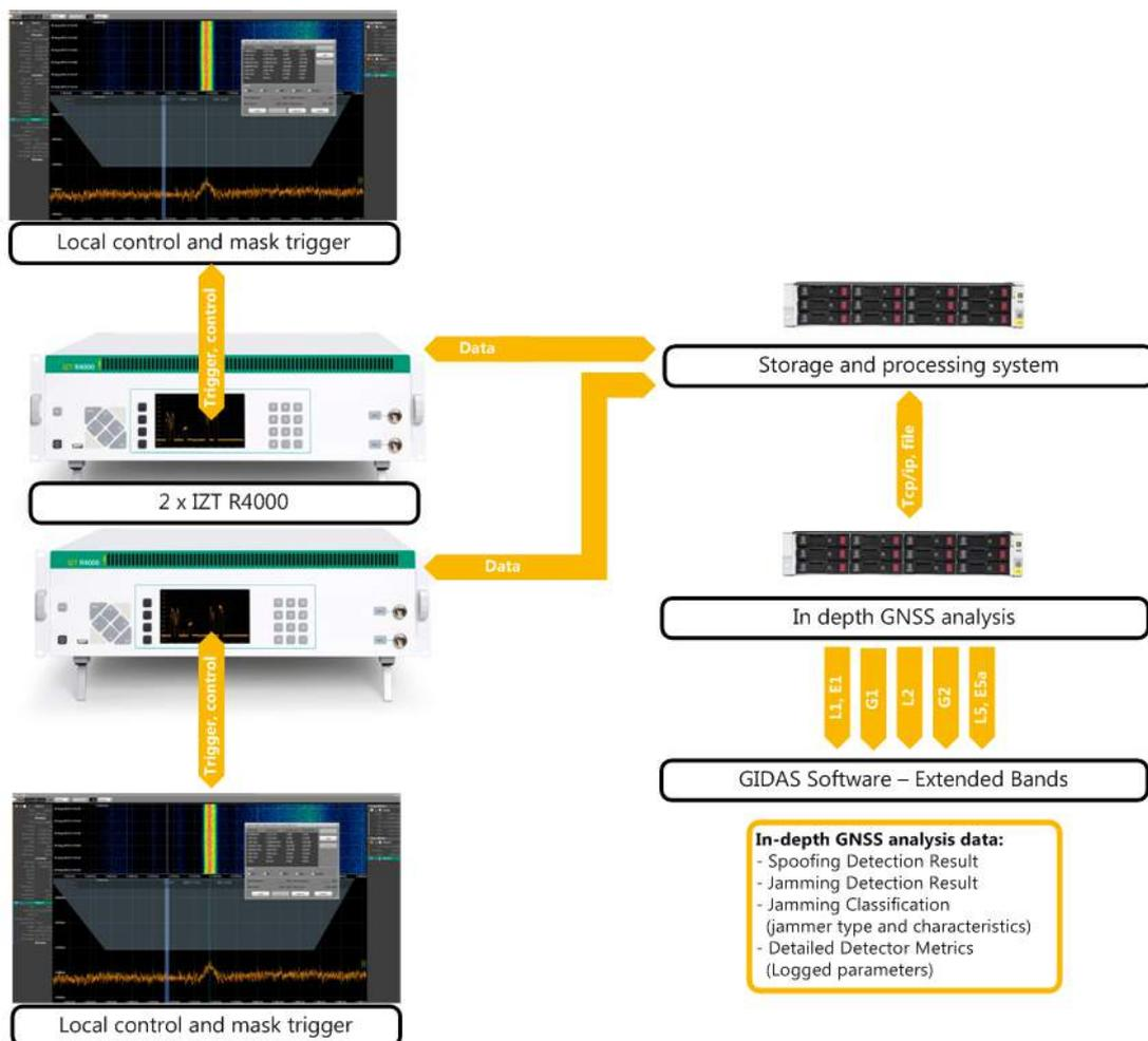
FIGURE 13: IZT GNSS MONITORING SYSTEM CONFIGURATION “C”
