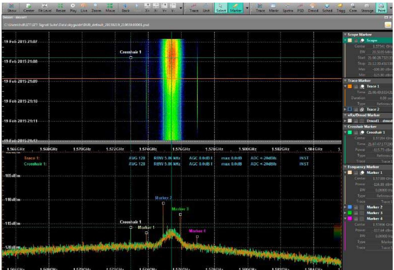
FIGURE 15: GNSS INTERFERER ANALYSIS WITH OFF-LINE APPLICATION IZT VIEWER
