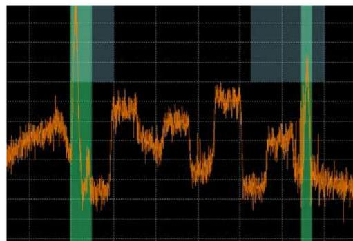
FIGURE 6: SELECTIVE TRIGGER ON SIGNAL EVENTS
