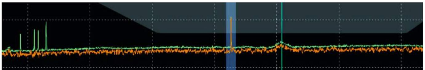
FIGURE 3: ONE INTERFERER MEETING MASK CRITERIA IS DETECTED AND TRIGGERS THE RECORDING TASK
