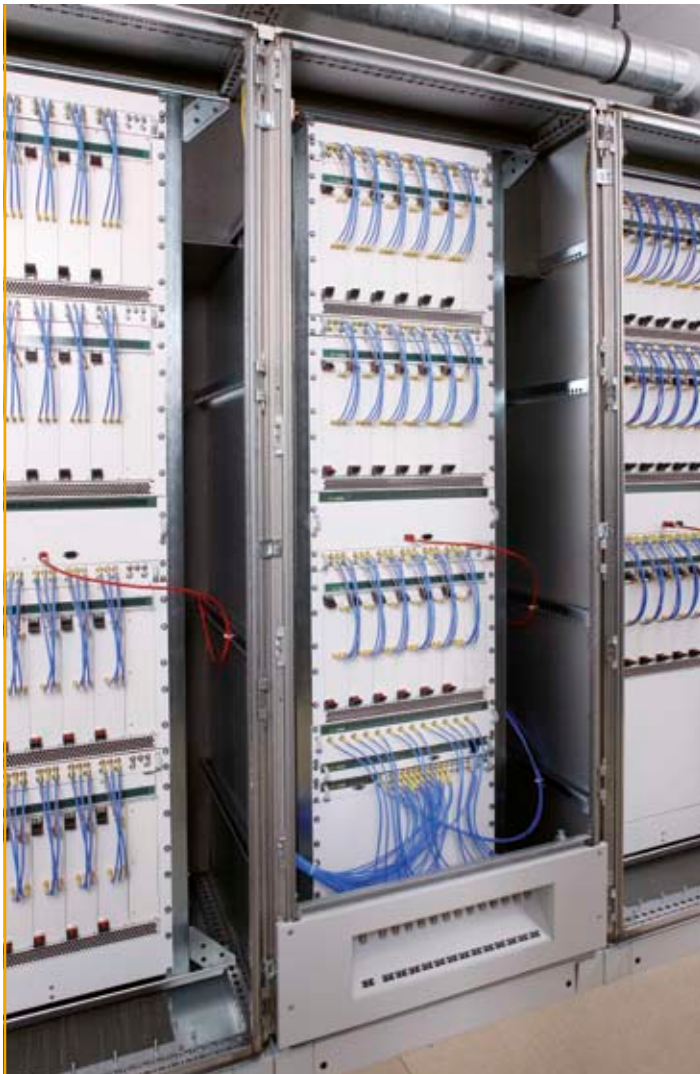
FIGURE 4: IZT S5000 IN A LARGE INSTALLATION FOR COMINT STIMULATION
