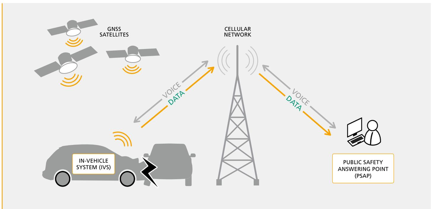
**FIGURE 2:** FUNCTIONALITY OF ECALL UNITS.
