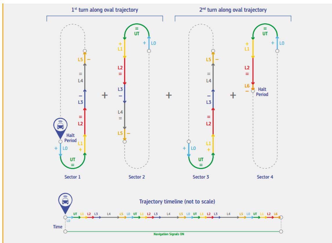
**FIGURE 5:** SKETCH OF A POSSIBLE OPEN-SKY VEHICLE TRAJECTORY TO BE USED IN THE DYNAMIC SCENARIO SPECIFIED IN SECTION 2.2.3 OF ANNEX VI [1], AND THE ASSOCIATED TIMELINE INDICATING THE TIME SERIES OF ALL THE TRAJECTORY SECTORS INVOLVED; © GSA/JRC
