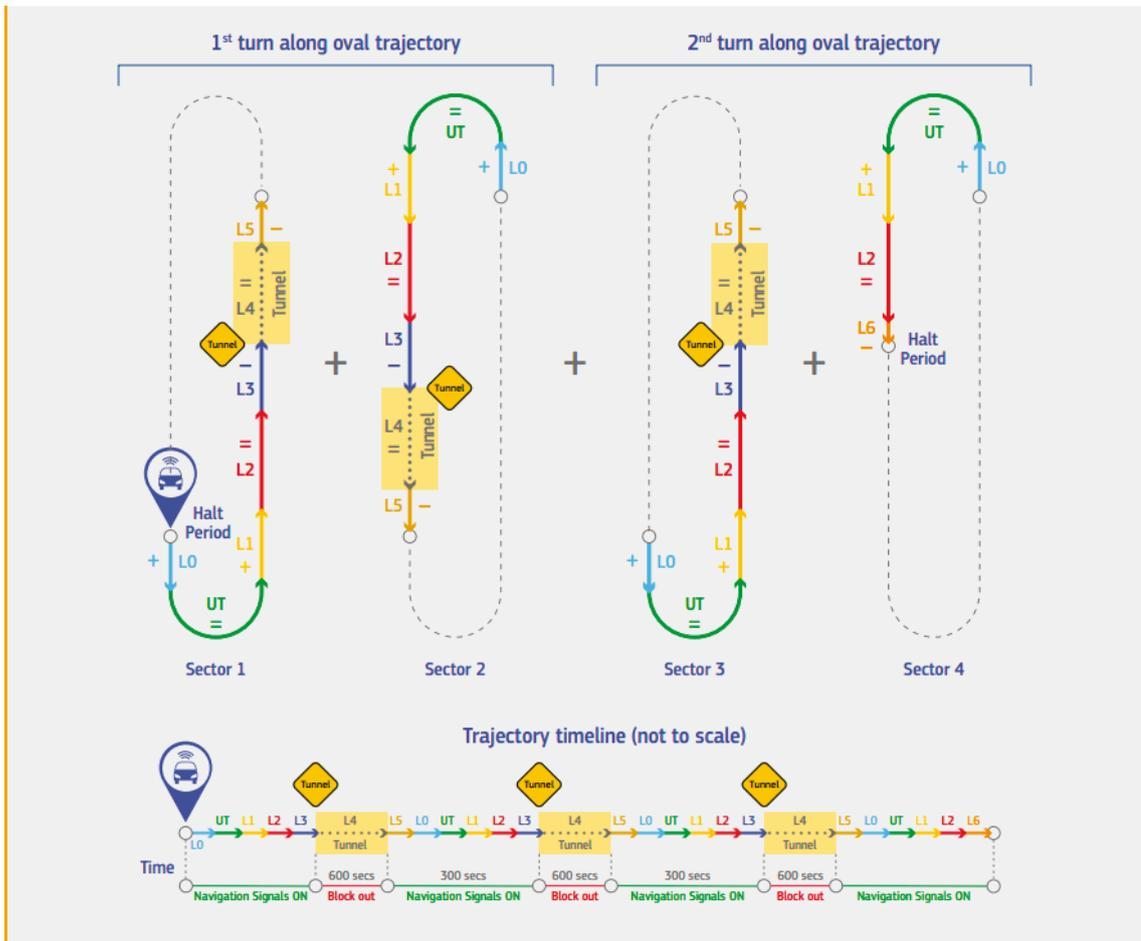
FIGURE 6: SKETCH OF A POSSIBLE OPEN SKY VEHICLE TRAJECTORY TO BE USED IN THE DYNAMIC SCENARIO SPECIFIED IN SECTION 2.2.4 OF ANNEX VI [1], INCLUDING THREE INTERVALS WITH A COMPLETE OUTAGE OF NAVIGATION SIGNALS, AND THE ASSOCIATED TIMELINE INDICATING THE TIME SERIES OF ALL THE TRAJECTORY SECTORS INVOLVED; © GSA/JRC
