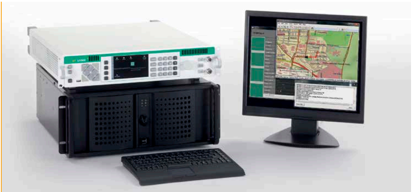
FIGURE 10: IZT S1000 REPLAY SETUP WITH IZT S1000 MEMORY EXTENSION+ STREAMING SERVER AND REAL-TIME GPS MAP VISUALIZATION
