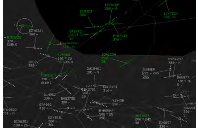
FIGURE 8: DETAIL OF A CONTROLLER'S SCREEN WITH A CIRCLE INDICATING THE LOCATION OF THE TRANSMITTING AIRCRAFT ©EUROCONTROL
