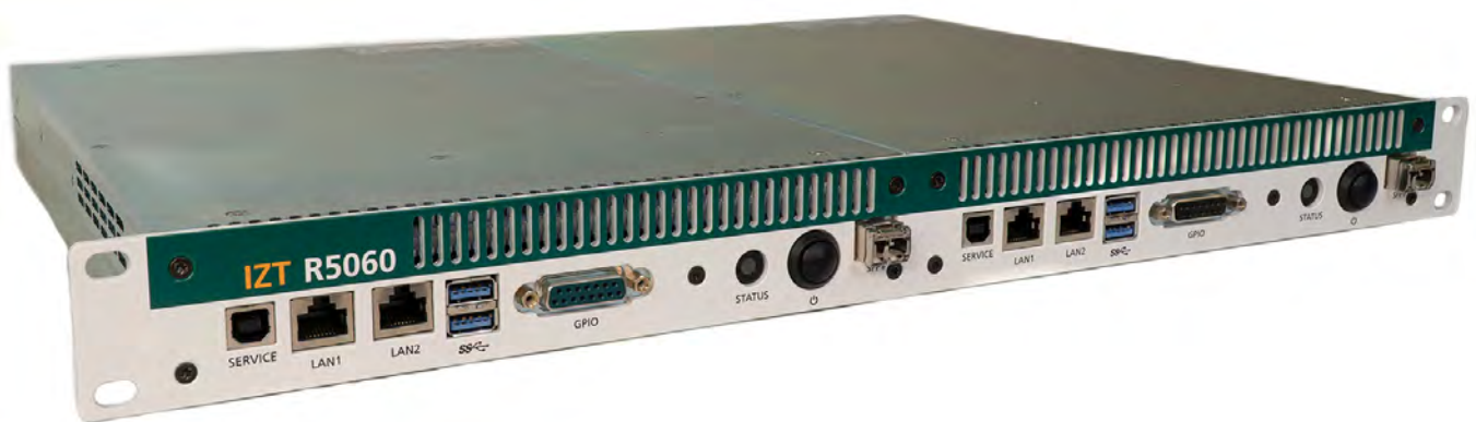
Figure 4: Two receivers installed in rack mount kit R5060-MNT with 1U form factor
