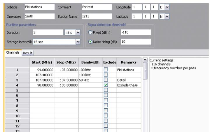
FIGURE 5: CONFIGURATION OF SPECTRUM OCCUPANCY MEASUREMENTS (DETAIL)
