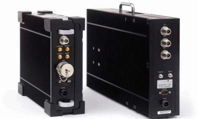
The compact variant of the successful R3000 series combines a limited weight of under 7 kg with a fanless design suited for harsh environments while maintaining the excellent HF performance and a real-time bandwidth of 24 MHz.
