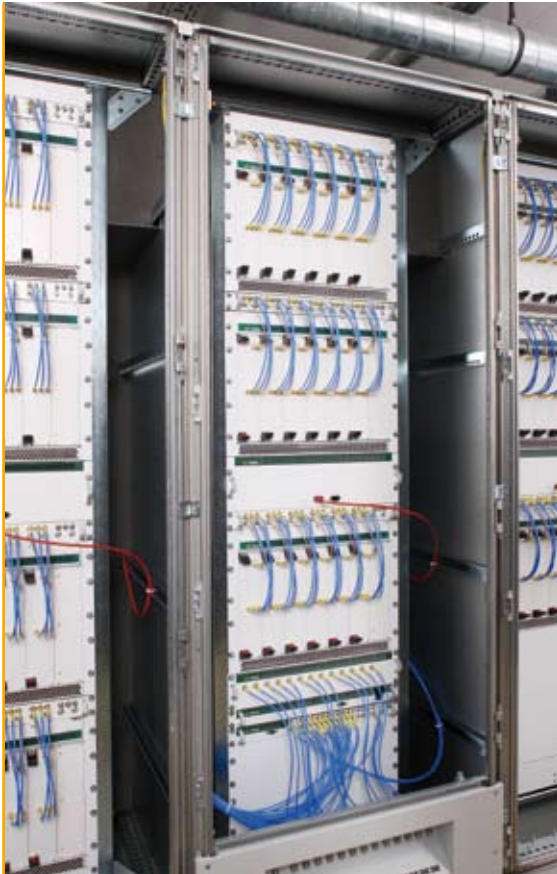
figure 3: IZT S5000 in a large installation for COMINT stimulation
