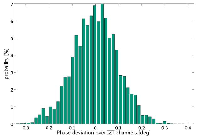
FIGURE 4: PHASE DRIFT HISTOGRAM
