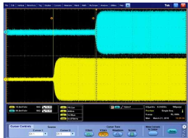
FIGURE 6: VERY LOW INPUT TO OUTPUT DELAY
