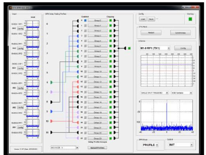
FIGURE 16: BPM GUI FOR CONFIGURING SWITCH MATRIX
