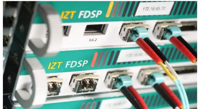
**FIGURE 7:** SIGNAL ROUTING VIA 10 GBIT ETHERNET
