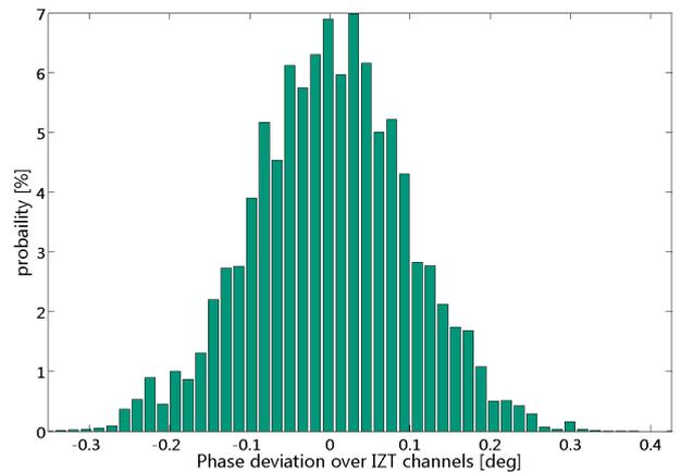
FIGURE 4: PHASE DRIFT HISTOGRAM
