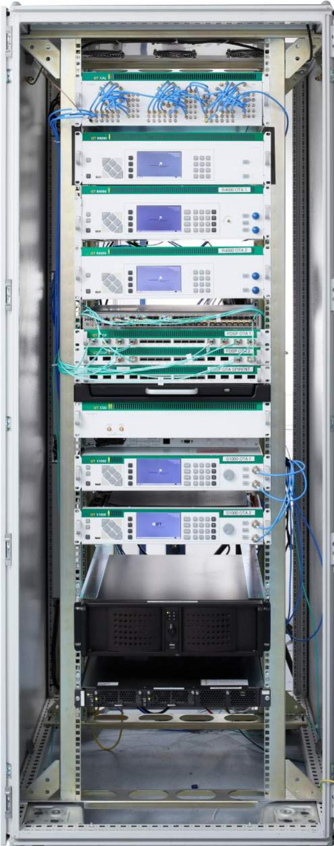
The IZT C7000 is a high-performance MIMO Simulator for the frequency range of 30 MHz to 6000 MHz with 80 MHz instantaneous bandwidth. The very low and adjustable input to output latency enables efficient testing of modern communication systems. The digitized signals are sent to the FPGA processor via optical cables to avoid loss of performance due to coaxial cables.
