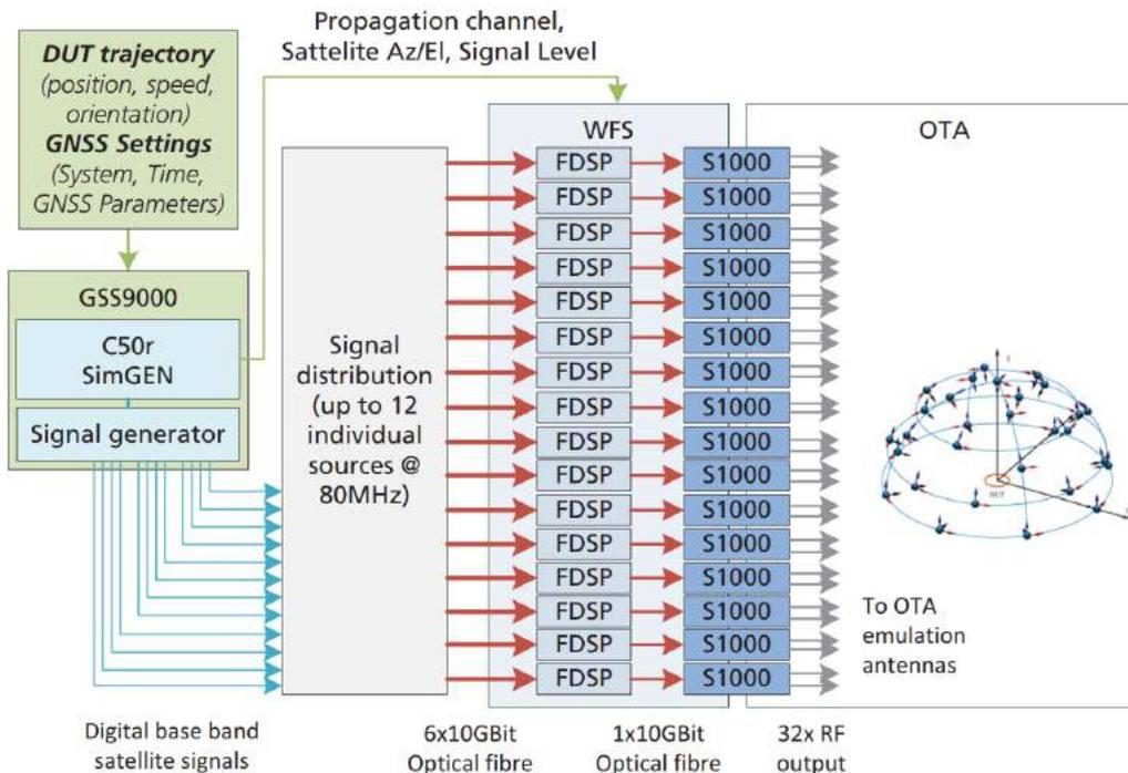
FIGURE 13: CUSTOMER INSTALLATION OF GNSS OVER WFS
