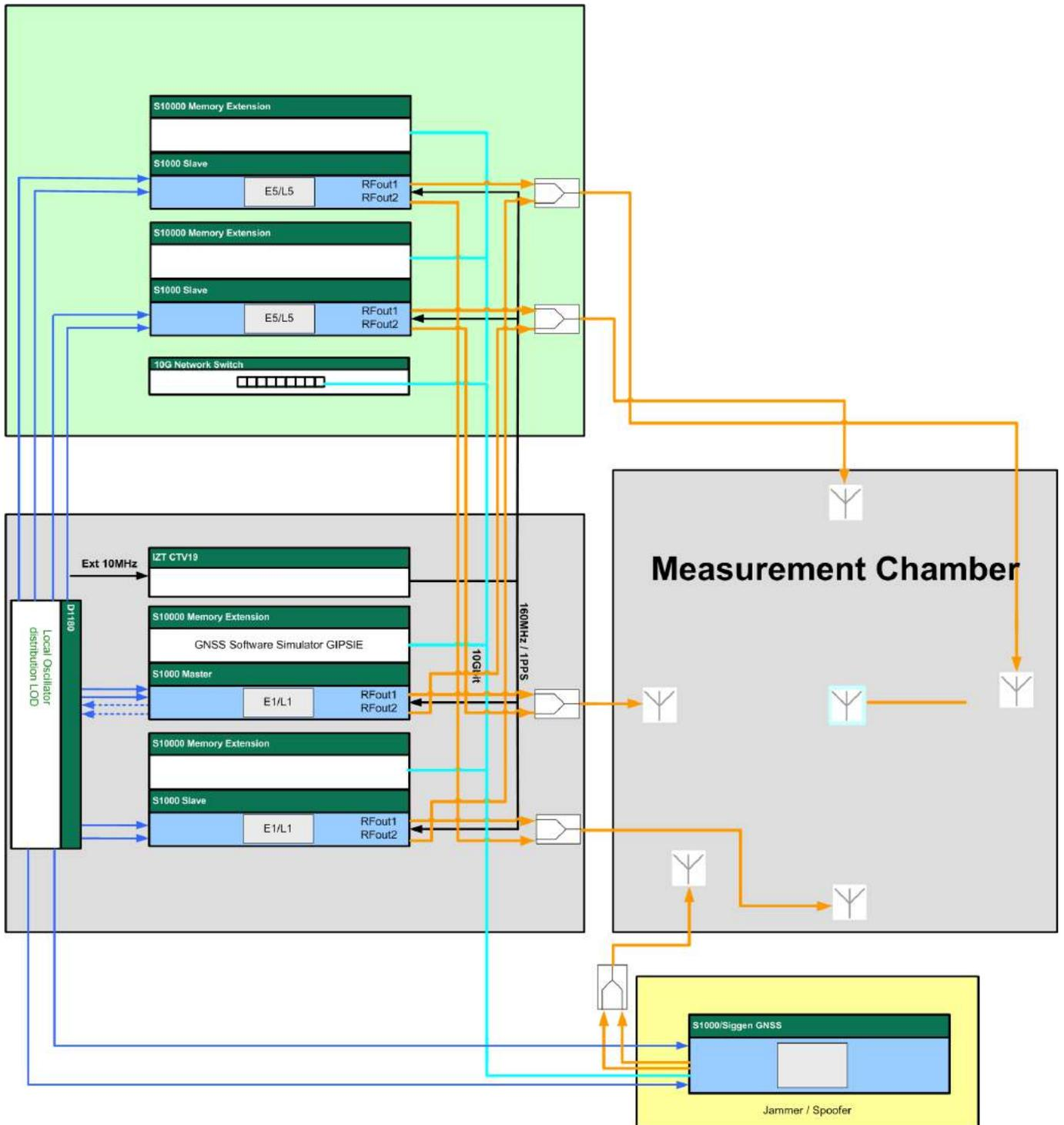
FIGURE 15: BLOCKDIAGRAM 4+1 L1/E1 L5/E5 ANTENNA SYSTEM
