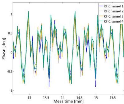
FIGURE 3: PHASE DRIFT OVER MULTIPLE RF OUTPUTS
