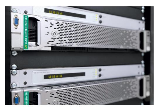
The IZT DAB ContentServer is in operation for a number of DAB ensembles performing encoding and multiplexing. It is operated on reliable IT server hardware and can be configured with a web interface.
