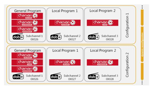
The change between different allocations of programs to DAB+ subchannels is performed as dynamic reconfiguration accordgin to the DAB standard.
