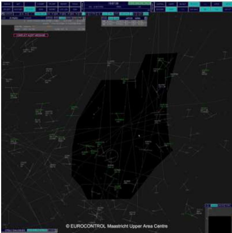
The currently speaking aircraft is shown in a circle on the control screen.
