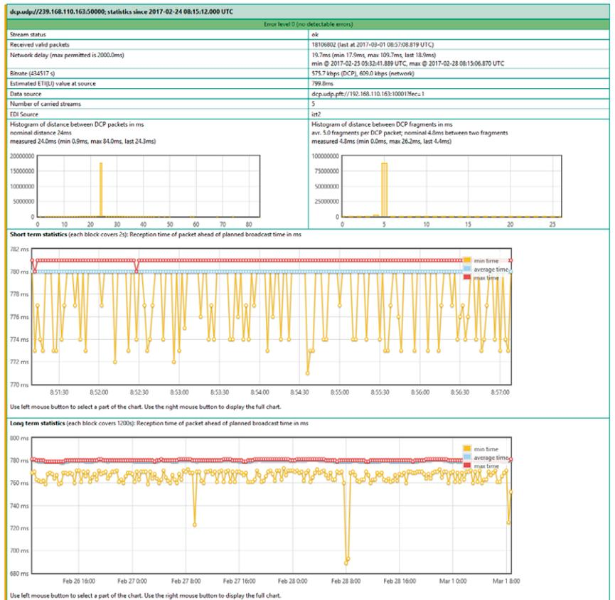
FIGURE 6: THE DCP MONITOR OF THE DAB CONTENTSERVER ALLOWS MONITORING OF INCOMING AND OUTGOING STREAMS
