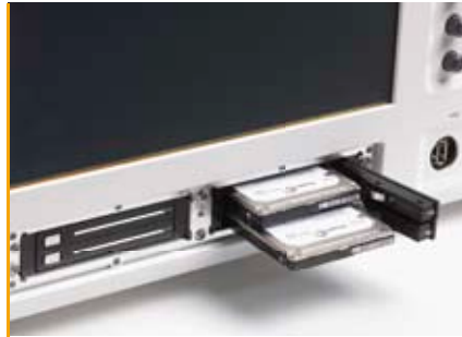
figure 5: Easy RAID storage swapping
