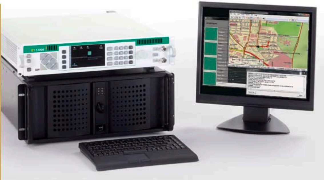
figure 10: IZT S1000 replay setup with P1200 streaming server and real-time GPS map visualization
