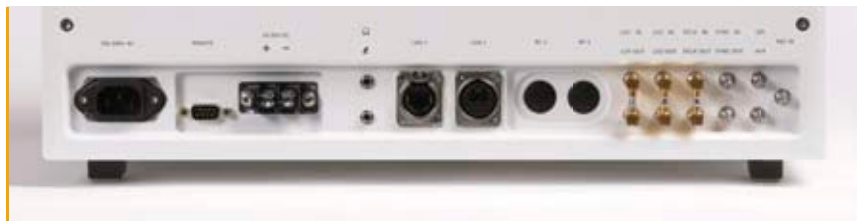
figure 7: External interfaces for power supply, LAN, GPS antenna and synchronization
